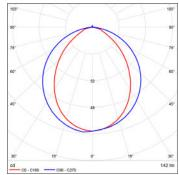
Polar curve for 600 lumen LED strip with opal diffuser.
