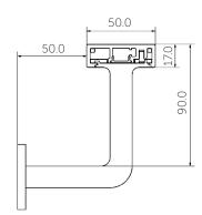
Richie Rail 17 is a unique illuminated handrail system. CNC machined wall brackets provide a beautiful finish and make for quick installation. Hollow wall brackets conceal the power supply to the LED strip, and the low voltage input makes the handrail safe to touch. Richie Rail 17 is suitable for use on residential and commercial stairs and thoroughfares.
