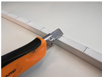
1. Cut through silicon casing at marked locations
