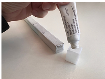
9. Use neutral-cure silicon to affix non-feed end cap at opposite end
