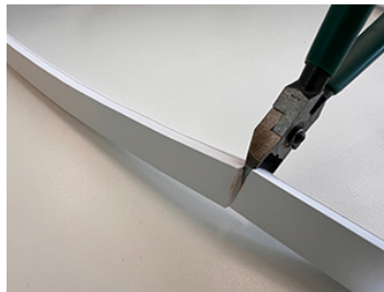
3. Use sharp side cutters to cut through PCB
