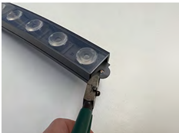
5. Trim internal plastic structure flush with end
