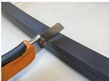
1. Cut through silicon casing at marked locations
