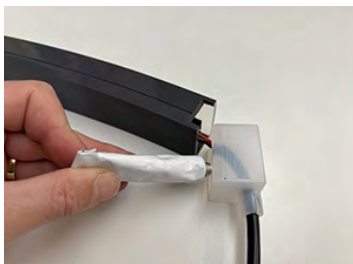
9. Fill end cap with neutral-cure silicon
