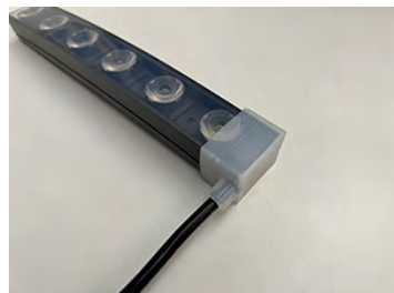
10. Finished feed end
