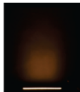
30° front view Distance to wall = 300mm Graze height on wall = 3800mm
