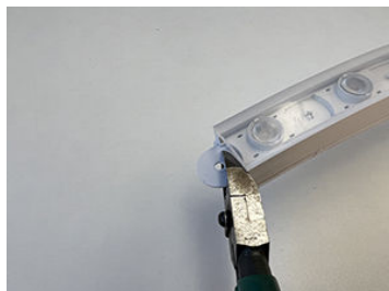
5. Trim internal plastic structure flush with end
