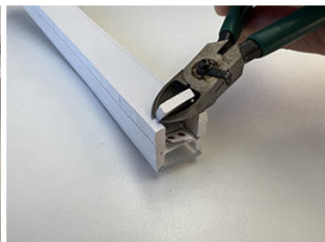
6. Trim silicon casing approx. 8mm from end as shown to allow cable to pass through
