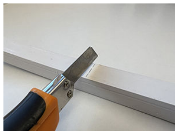
1. Cut through silicon casing at marked locations
