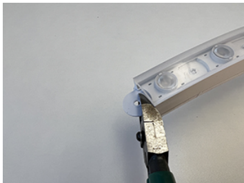
5. Trim internal plastic structure flush with end
