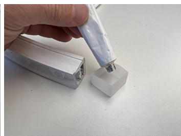
11. Use neutral-cure silicon to affix non-feed end cap at opposite end
