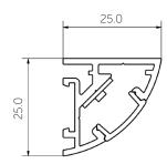
The Angle Andy 25 profile is perfect for mounting in corners of joinery, corners of perpendicular walls or into the corner of a wall and ceiling. Angle Andy 25 features one smooth side, meaning it is not confined to corner mounting, but can also be mounted with one side of the extrusion visible - ideal for wall washing or glass cabinetry.
